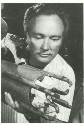
Spark gap drilling bit
